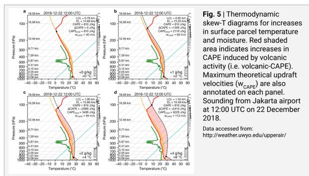
**Fig. 5 |** Thermodynamic skew-T diagrams for increases in surface parcel temperature and moisture. Red shaded area indicates increases in CAPE induced by volcanic activity (i.e. volcanic-CAPE). Maximum theoretical updraft velocities ( $w_{CAPE}$ ) are also annotated on each panel. Sounding from Jakarta airport at 12:00 UTC on 22 December 2018. Data accessed from: <http://weather.uwyo.edu/upperair/>
