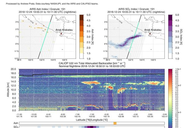
**Supplementary Fig. 1 |** CALIOP/AIRS analysis<sup>2</sup>. Black line with green highlight indicates CALIOP track over AIRS ash/SO<sub>2</sub> detection track indices (top panels). UTLS volcanic feature present in CALIOP backscatter curtain (lower panel).
