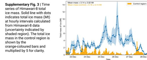
**Supplementary Fig. 3 |** Time series of Himawari-8 total ice mass. Solid line with dots indicates total ice mass (Mt) at hourly intervals calculated from Himawari-8 data (uncertainty indicated by shaded region). The total ice mass in the control region is shown by the orange-coloured bars and multiplied by 5 for clarity.
