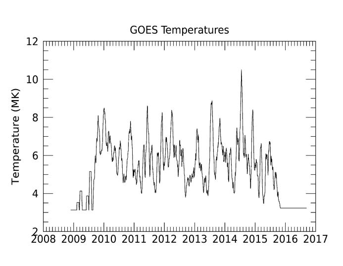
Knowledgebase (HEK), we can calculate the quiet coronal temperatures, which dominate the full-disk measurements and change with solar cycle.
