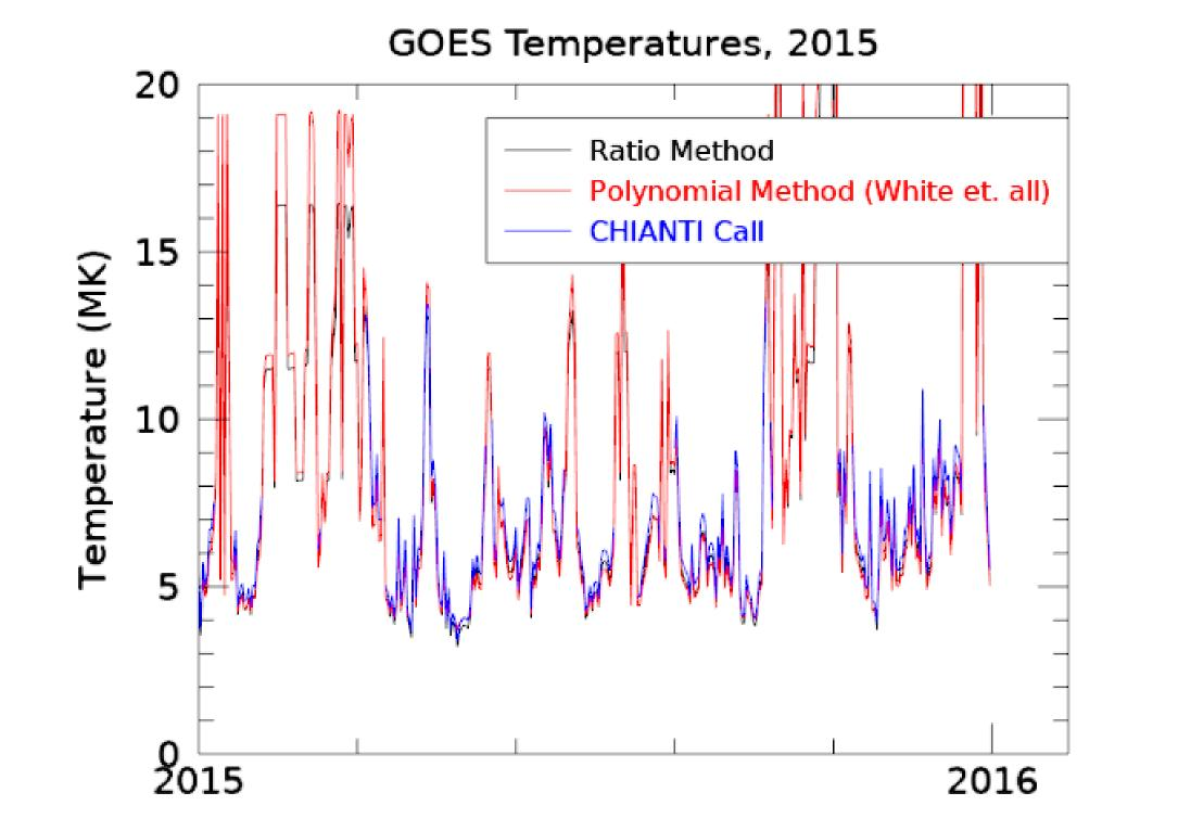
Based on MINXSS and GOES data, hot plasma during the most recent solar cycle appear to hold steady at a temperature of about 6.4 MK. Using the assumption that the active corona plasma is relatively constant and incorporating active corona area information from the Heliophysics Events
