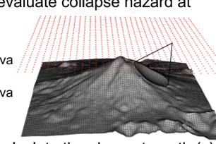
Scoops3D applies the Coulomb failure criteria to calculate the shear strength (s)
