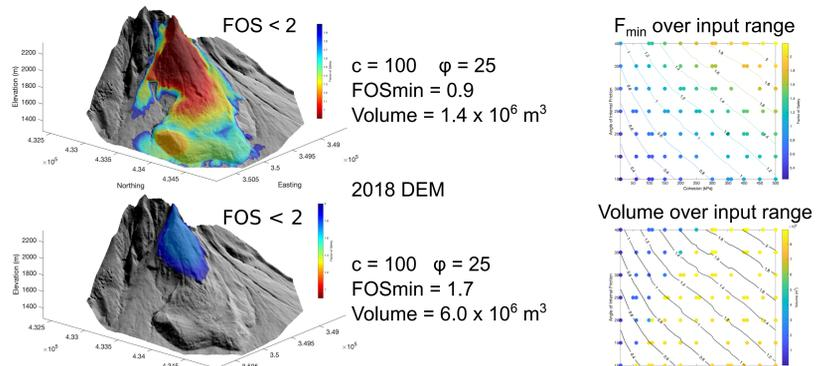
Accurate constraint of material properties is essential for assessing the FOS of a failure surface. However, the location and volume of the surface where FOS<sub>min</sub> occurs is not strongly affected by the material properties.
