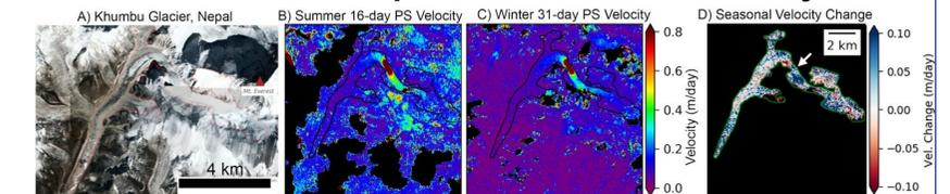
Figure 7: Seasonal velocity for Khumbu Glacier derived from corrected PS 3-m orthoimages with 16-day and 31-day separation for June-July (summer) (B) and October-November (winter) (C), respectively (arrow in D highlights seasonal change below/above fast-flowing region of Khumbu icefall).
