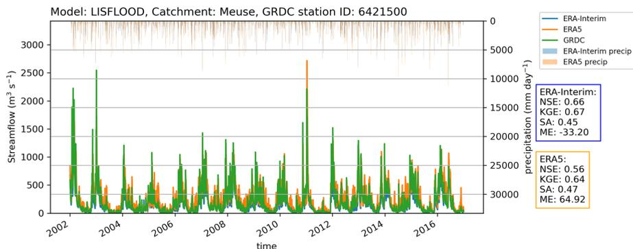
Example output from the LISFLOOD model for the Meuse
