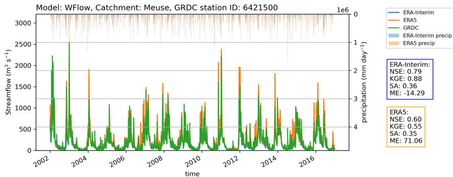
Example output from the WFLOW SBM model for the Meuse
