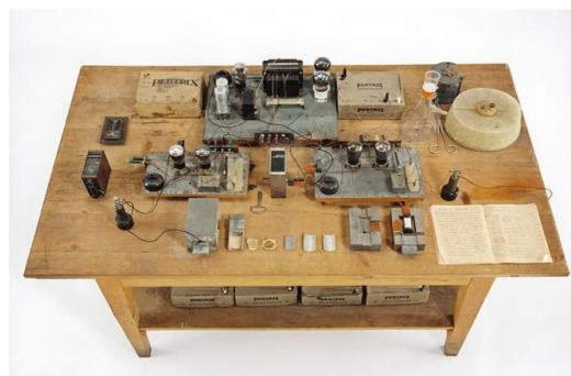
Copy of first nuclear fission experiment. On the right, you see a source of fast neutrons (a radium and beryllium mixture) in a hydrogen-rich block of paraffin. The paraffin slowed down the neutrons so they could be "absorbed" by uranium nuclei, which then became unstable and split into barium and krypton. Similarly, we moderate fast neutrons so they can be captured by ^{10}\text{B} .
