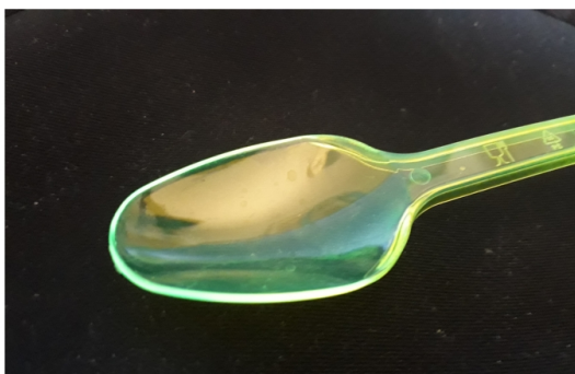
Wavelength shifting fibers are not unlike ice-cream spoons. Green light has a relatively large internal angle of reflection and the spoon becomes a wave-guide. A large number of photons come out at the edge, as if there is an internal light source. We call this the dicula effect.
