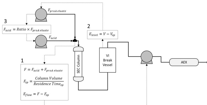
Figure 7. Schematic of mass flow rate control. (1)  $F_{proA eluate}$ : protein A product material flow rate,  $F_{acid}$ : acid flow rate,  $F$ : total flow into VI SEC column,  $F_{sp}$ : set point flow rate,  $E_{flow}$ : error in target flow into SEC column. (2)  $E_{level}$ : Error in target vessel level,  $V$ : vessel level,  $V_{sp}$ : set point vessel level. (3) Ratio: target ratio of acid flowrate to product flowrate.
