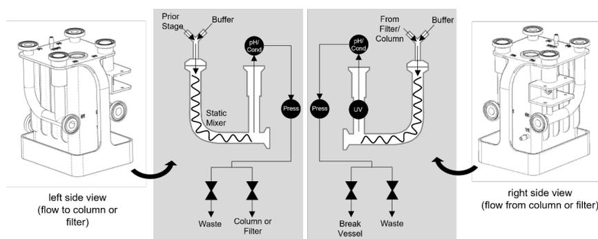
Figure 2. Flow path of the PAK single-use flow kit for individual process steps (chromatography, virus inactivation, membrane, filtration). Includes pH, conductivity (Cond), and pressure (P) instrumentation.
