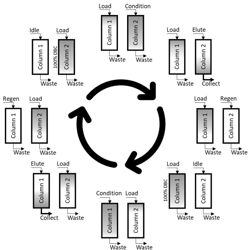
Figure 3. Diagram illustrating the dual column operation. Condition indicates pre elution phases such as equilibration and wash. Regen indicates the combination of the post-elution phases: strip, sanitization and
