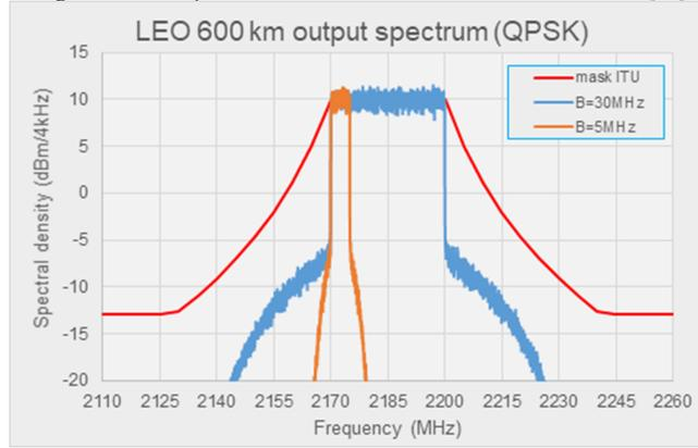
Fig. 15. Out-of-Band Spectrum with respect to the Percentage of SAN Bandwidth [23]
