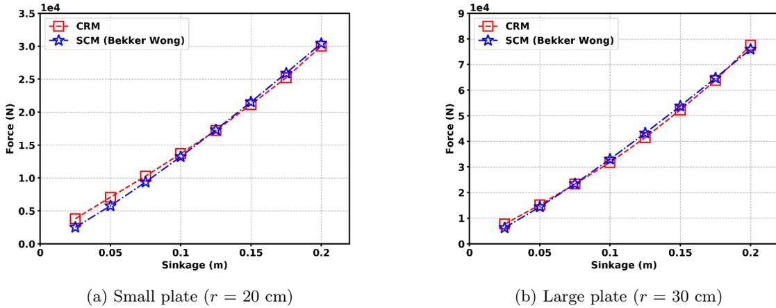
Figure 9: A comparison between selected points using CRM model and SCM model. The SCM results are calculated using calibrated values of  $K_c$ ,  $K_\phi$ , and  $n$  and the Bekker-Wong formulation in Eq. (1).
