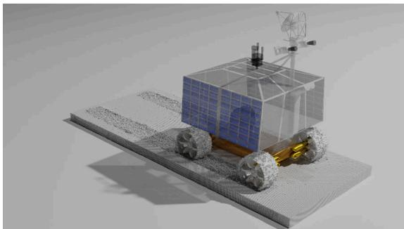
Figure 29: Rover positions and SPH particle distributions of the terrain with different wheel slips modeled using CRM approach.
