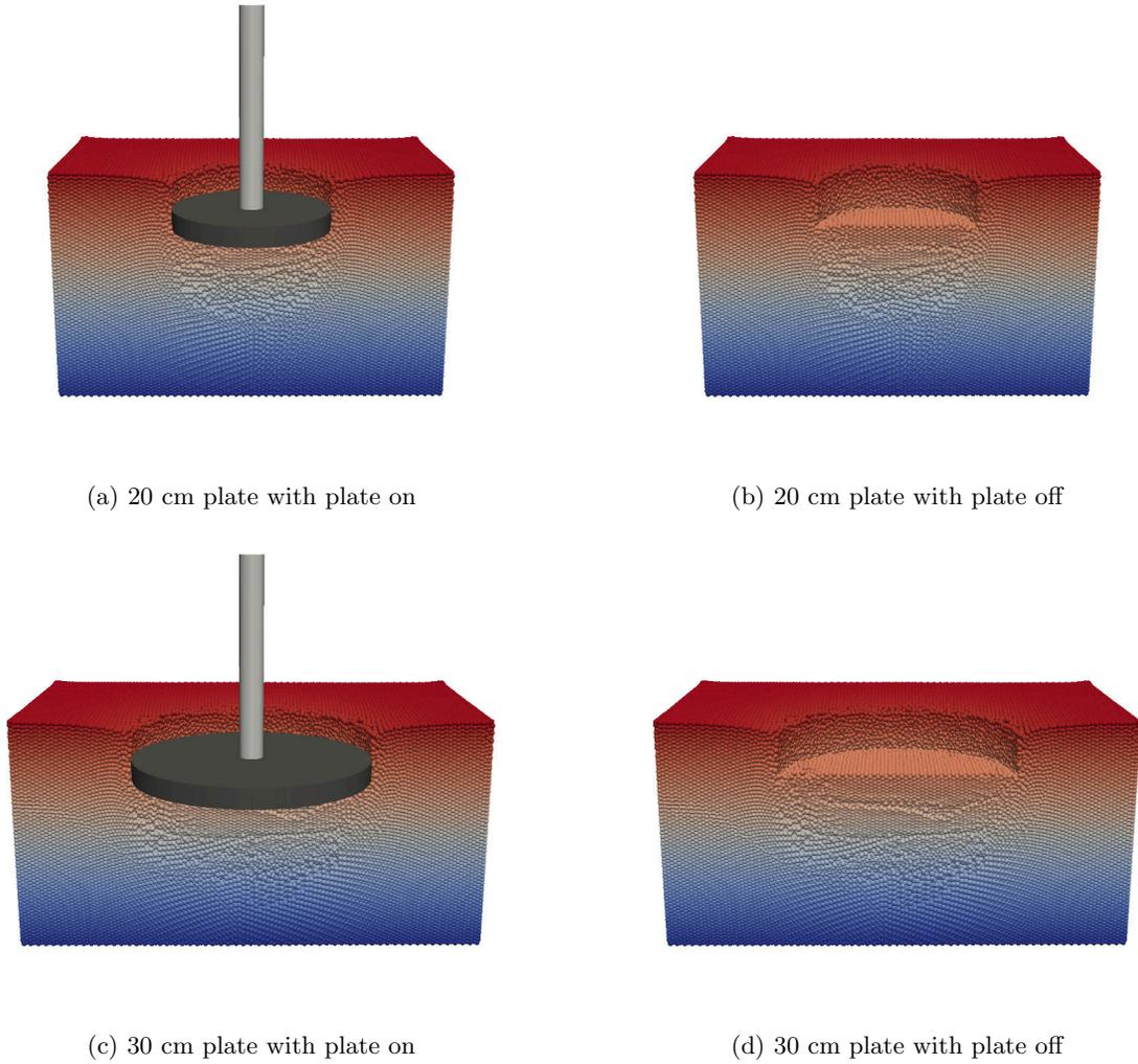
Figure 1: Plate sinkage tests using the virtual bevameter with different plate sizes; the vertical speed was constant during each test.
