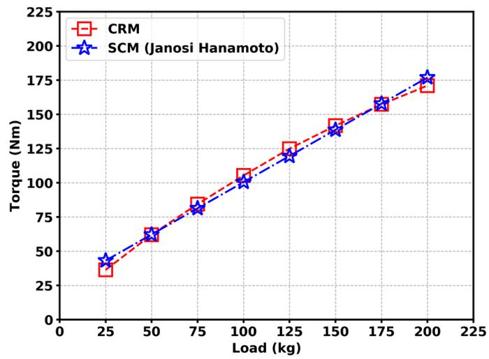
Figure 18: A comparison between selected points using CRM model and SCM model. The SCM results are calculated using calibrated values of  $c$ ,  $\varphi$ , and  $K_s$  and the Janosi formulation in Eq. (3).
