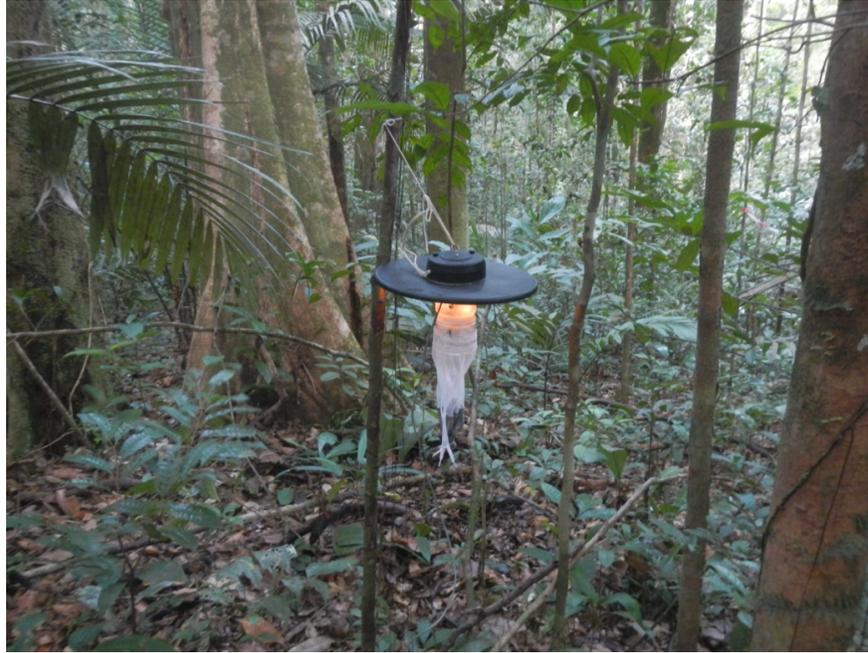
Figure 2: Light trap used for the collection of phlebotomine sand flies (credit: A. Kocher)
