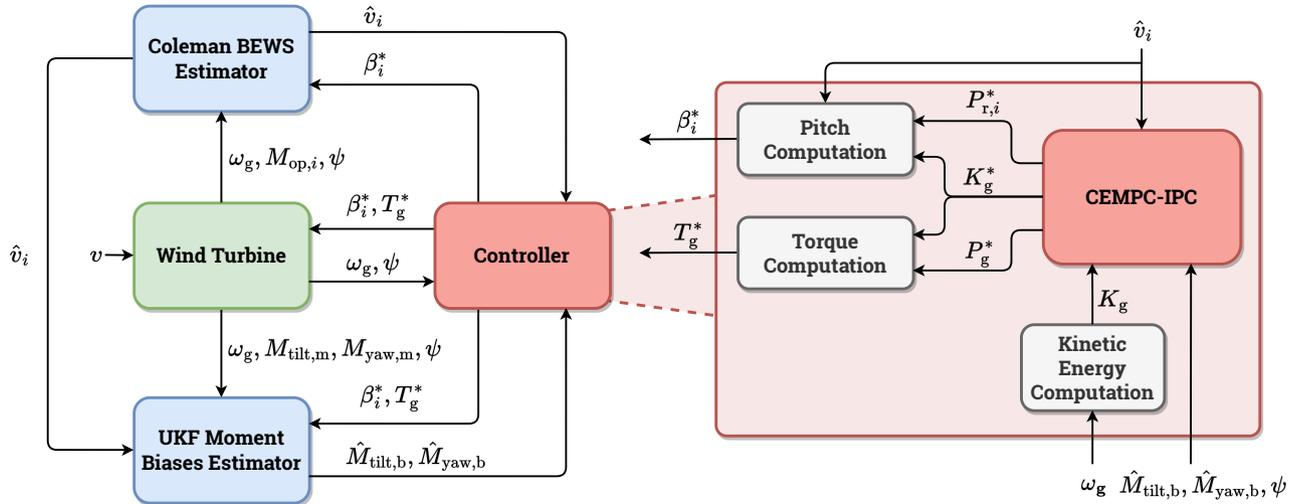
**FIGURE 2** CEMPC-IPC implementation setup. A blade-effective wind speed (BEWS) and moment biases estimator via unscented Kalman filtering (UKF) are included for providing unknown information to the controller.
