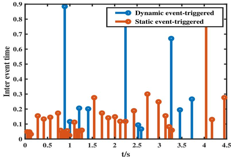
FIGURE 5 The event-triggered interval  $\{t_{k+1} - t_k\}$ .
