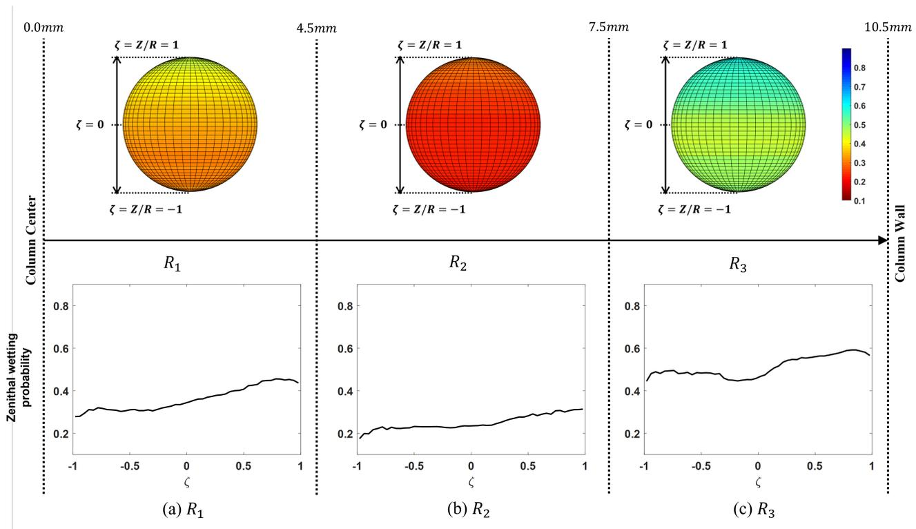
Figure 19: Zenithal wetting probability profile of the particles at the three radial sections:  $R_1$  (a),  $R_2$  (b), and  $R_3$ (c).
