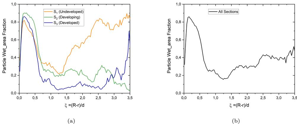
Figure 16: Radial particle wet area profile at the three different axial sections:  $S_1$ ,  $S_2$ , and  $S_3$  (a) and averaged over all the sections (b).
