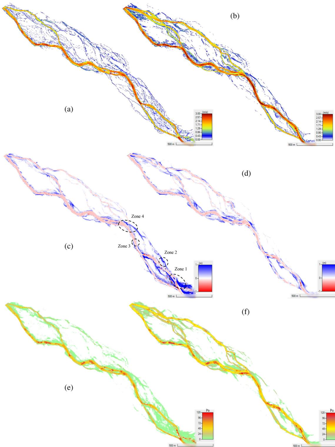
**FIGURE 10** Velocity, bed changes, and bed shear stress patterns of scenario with the regulated discharge hydrograph (a, c, and d, respectively), and for the scenario with the non-regulated discharge hydrograph (b, d, and f, respectively). [Color figure can be viewed at [wileyonlinelibrary.com](https://onlinelibrary.wiley.com/doi/10.1002/tra.4268)]
