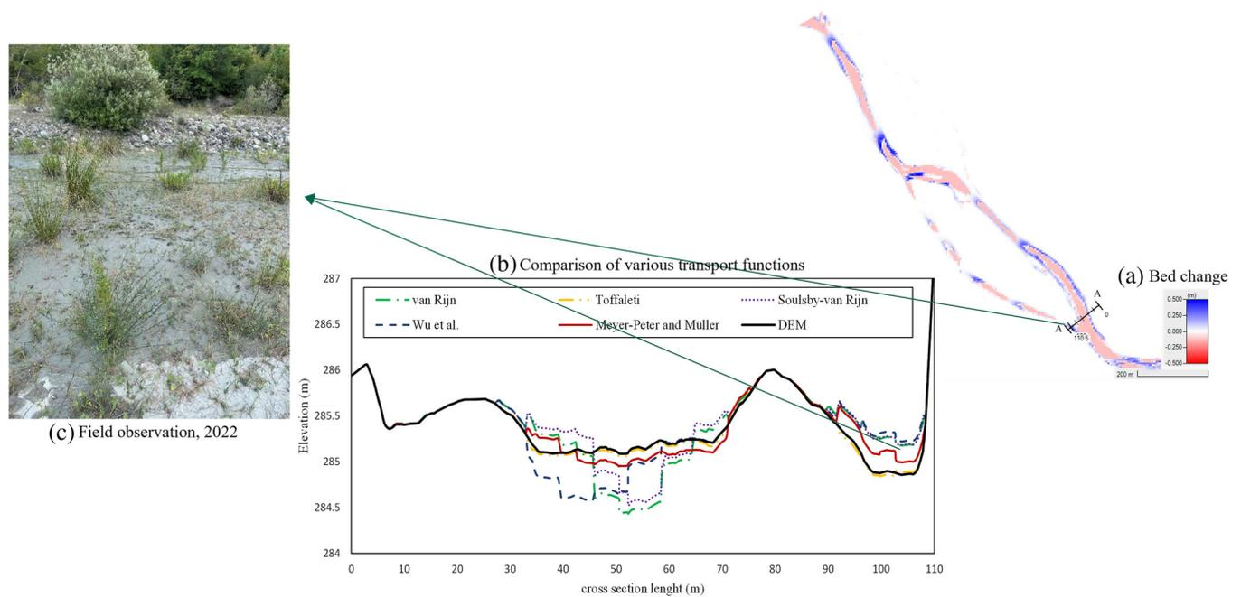
**FIGURE 7** (a) Bed change of a test with Meyer-Peter and Müller transport function, (b) comparison of various transport functions on section A-A, and (c) field observation in 2022. [Color figure can be viewed at [wileyonlinelibrary.com](http://wileyonlinelibrary.com)]
