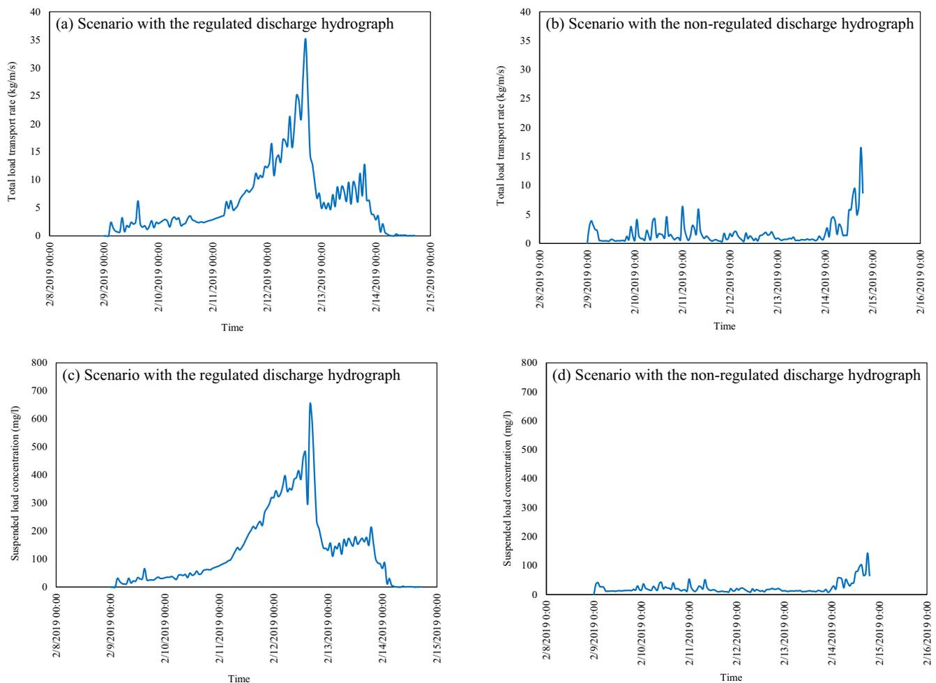
**FIGURE 11** Total load transport rate and suspended load concentration for both scenarios A and B. [Color figure can be viewed at [wileyonlinelibrary.com](http://wileyonlinelibrary.com)]
