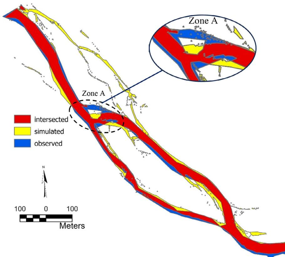
**FIGURE 6** Comparison of the simulated and observed water inundation areas for the test with Meyer-Peter and Müller transport function. [Color figure can be viewed at [wileyonlinelibrary.com](http://wileyonlinelibrary.com)]
