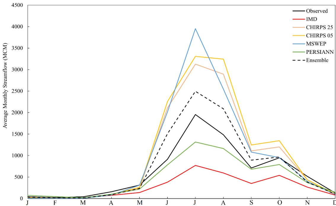
645 Figure 10 The monthly average streamflow in MCM at KRS simulated using the IMD,
