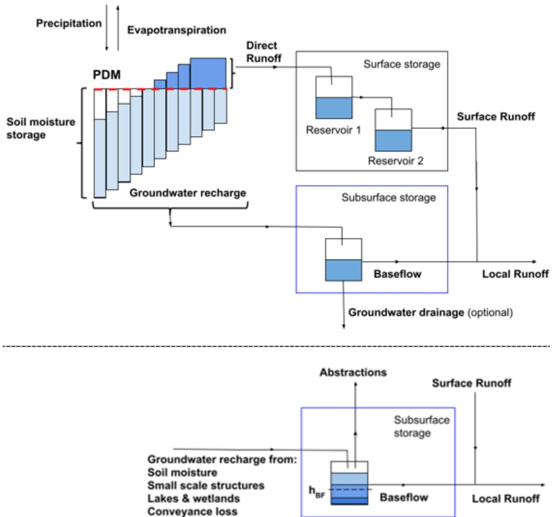
370 Figure 3 Schematic of the rainfall-runoff model, including the configuration of the probability
