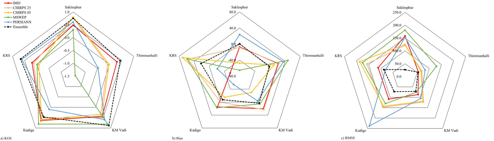
641 Figure 9 The monthly a) Kling-Gupta Efficiency (KGE) b) Bias in percentage and c) Root mean squared error (RMSE) of the simulated
