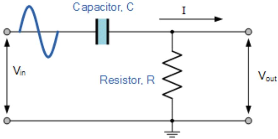
Figure 3: RC high pass filter
