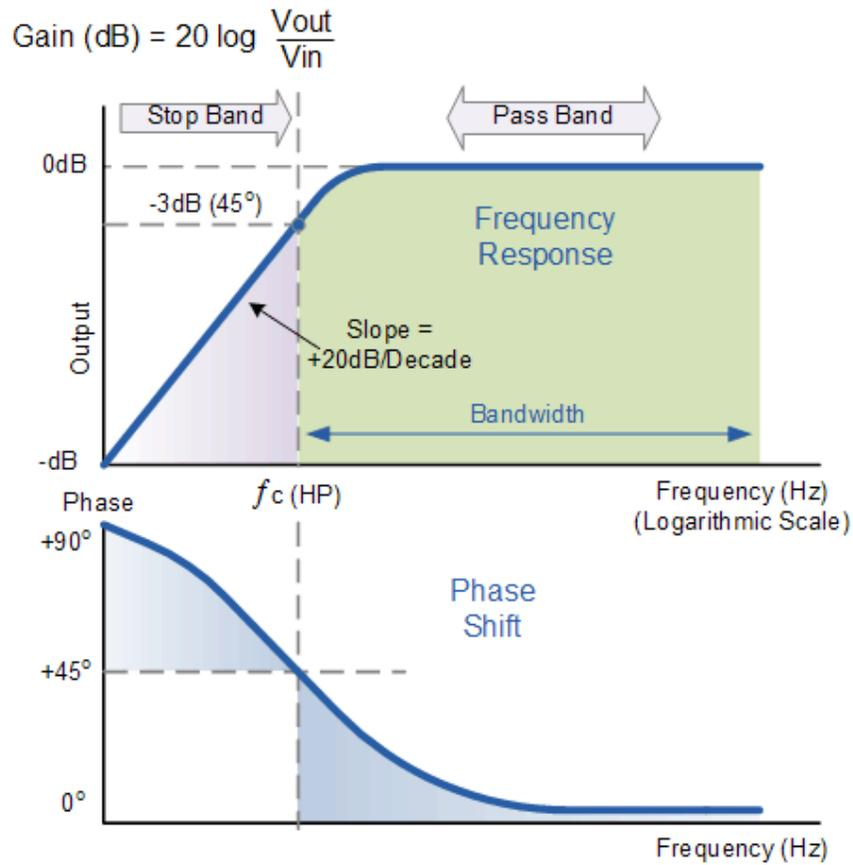
Figure 4: High pass filter amplitude and phase diagram
