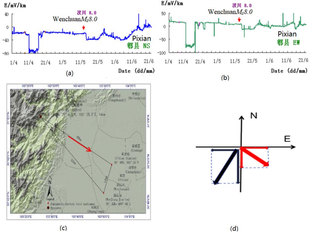
Fig. 3 The goelectric field orientation diagram before and after the Wenchuan earthquake based on Pixian station data[18]
